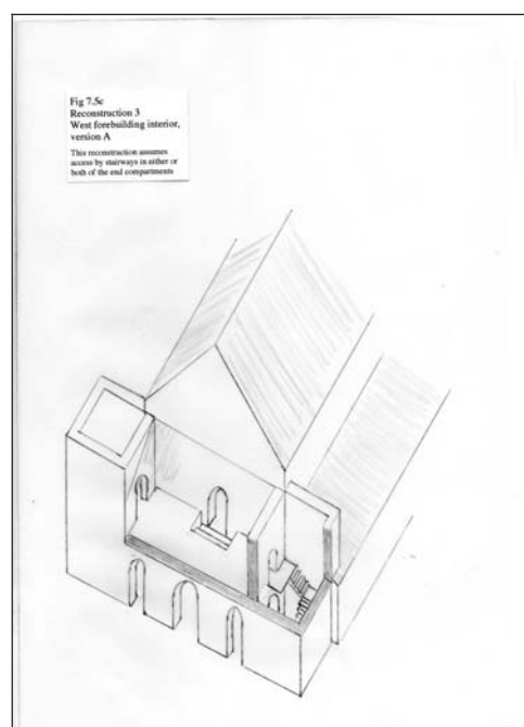
Suggested reconstruction of the western forebuilding; the cut-away view shows the postulated upper chamber and the approach stairs in the turriform end chamber (draft)
